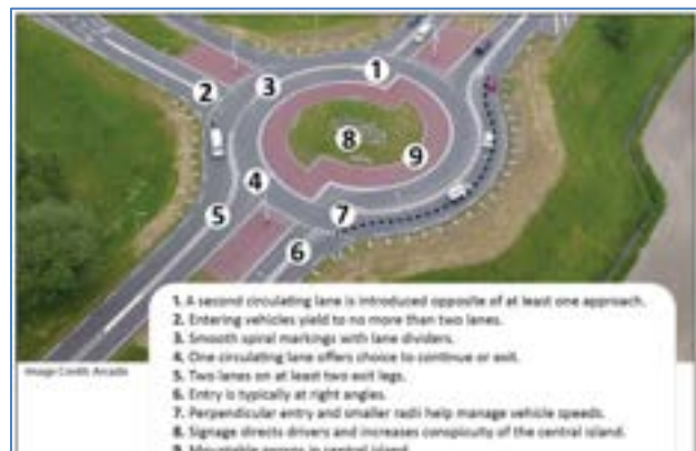
Characteristics of a typical Turbo Roundabout.
