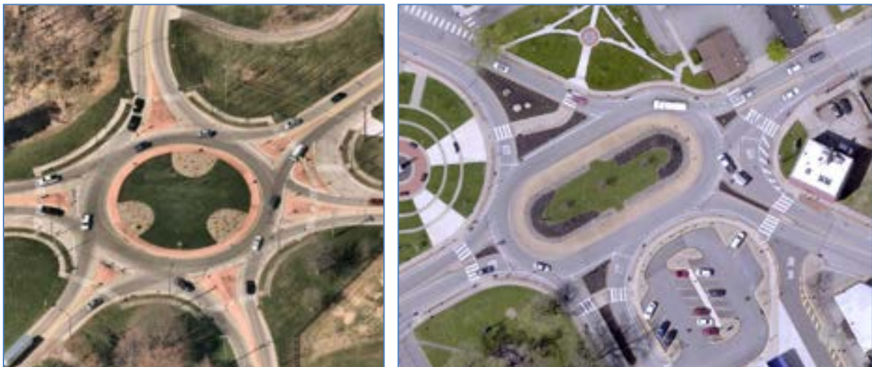
Examples of roundabouts with more than four legs—Left: The Northeast / Howe / N. Munroe roundabout in Tallmadge is among the largest roundabouts in the region; Right: This 5-leg elongated roundabout in Rochester, PA combines five high-volume roadways on the edge of the borough's downtown.
