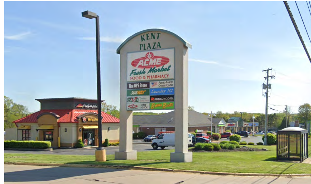
FIGURE 11 Bus shelter near Pizza Hut is accessible from the road/bus but there is no pedestrian access from the bus stop to the business entrance. A person in a wheelchair would be forced to navigate around the lawn by using the driveway, which would put them at risk.
