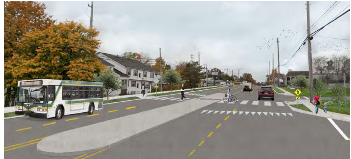
FIGURE 13 Proposed mid-block crossing with pedestrian island
