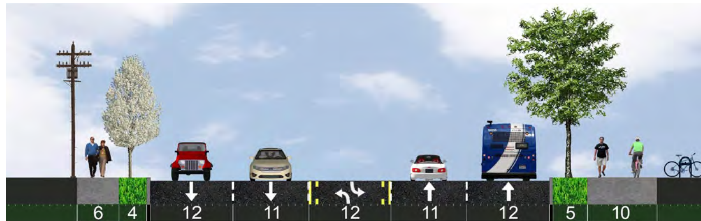
FIGURE 3 Proposed corridor right-of-way and lane widths
