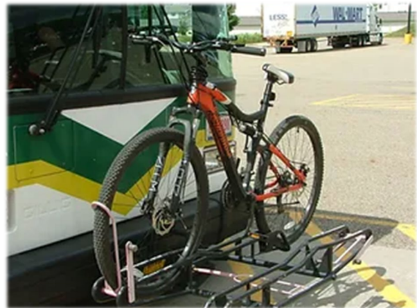
PARTA Bike Rack—This feature enables cyclists to attach their bikes easily and securely to the front of the bus, expanding travel options for those who rely on bicycles to reach specific destinations, nearby shared paths, or regional trail networks.
