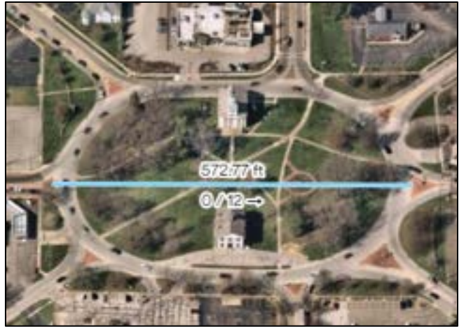
Two local examples of traffic circles, Mull/Hawkins (left) and Tallmadge Circle (right). Note the large, inscribed diameter of both circles.
