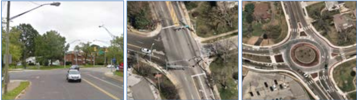
Local example of a roundabout improving the geometry of a previously skewed intersection (E. Market St. /Canton Rd. /Robindale Dr. in Akron). The two photos on left show the intersection before the roundabout was constructed; right photo showing the roundabout.
