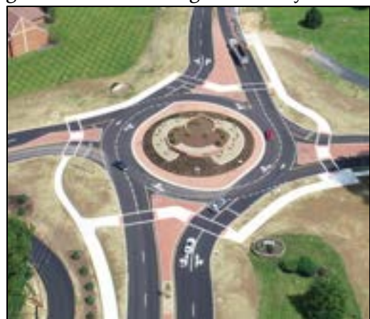
Regional Example of a suburban 2 x 1 roundabout located at Cleveland-Massillon/Rothrock in Fairlawn
