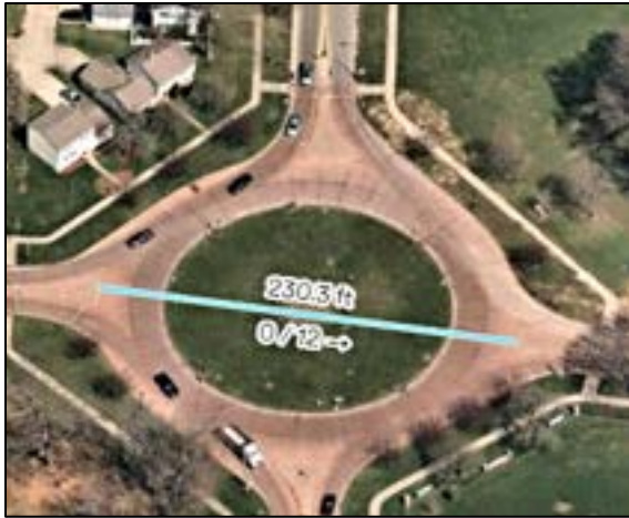
Two local examples of traffic circles, Mull/Hawkins (left) and Tallmadge Circle (right). Note the large, inscribed diameter of both circles.
